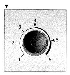
Position 1 gives the lowest light intensity, and maximum brightness is attained in position 6. The two barriers at positions 4 and 5 are bypassed by pressing in the adjustment knob.
