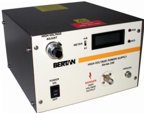
Spellman's Bertan brand of 230 Series high voltage power supplies provide regulated high voltage outputs from 1 to 30kV. The low noise, linear topology employed results in extremely low output ripple specifications. These 12 to 15 watt units are inherently reversible by design, providing either positive or negative output polarity. The 230 Series is fully arc and short circuit protected. Excellent regulation specifications are featured along with outstanding stability performance.
