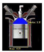
Stroke 1: The intake valve opens, and the piston moves down. This brings a mixture of air and fuel into the chamber.
