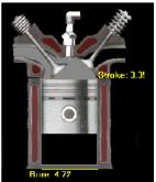
Stroke 3: The spark plug then initiates the combustion of the gas. The explosion pushes the piston down. The piston is connected to a crankshaft that delivers power to the drive train and the wheels.
