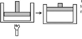
The flame on the right is turned on, which heats up the gas causing it to expand. The piston is connected to a drive train that causes a car to move. The signs of q and w for the gas in the cylinder are:
